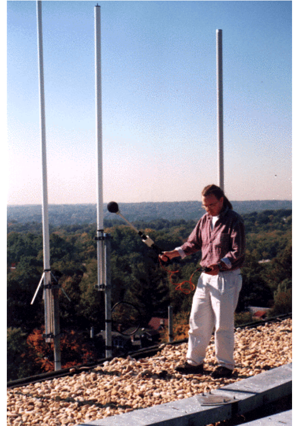
Site Survey to measure EME exposure as percentage of MPE
